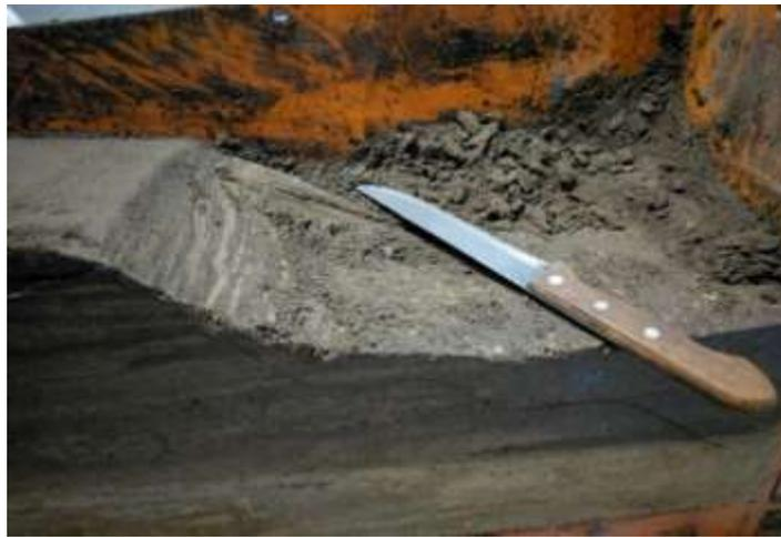
**Figure 3** Slicing the soaked soil according to the profile of the slope
