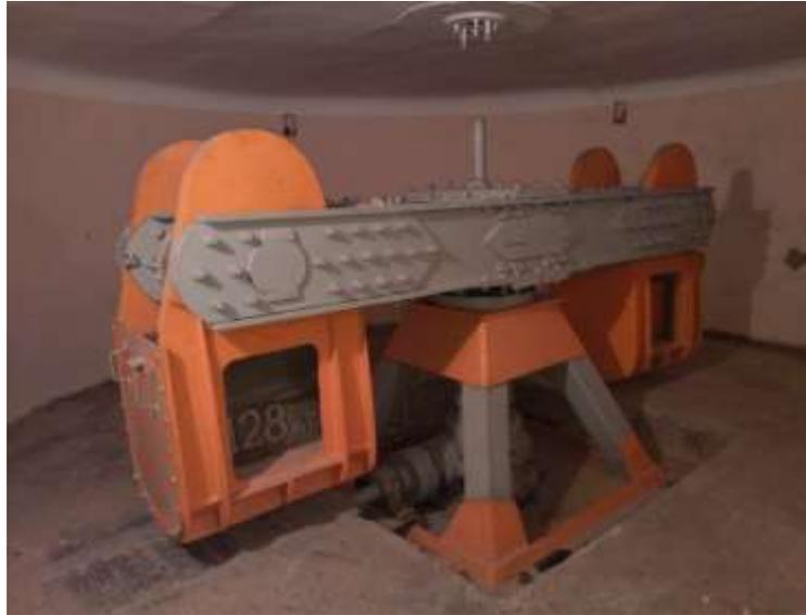
**Figure 1** The centrifuge was used to study the stability of the Krasnovpostanska ravine slope
