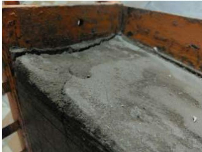
**Figure 5.** Creation of cracks and separation surfaces, drainage of soil after centrifuge rotation
