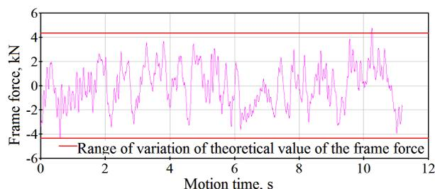
Fig. 9. Comparison of experimental values of the frame force acting in the diesel train car at a speed of 30 m/s in a straight railway track section with the values obtained in theoretical calculations
