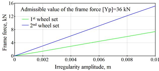
Fig. 3. Dependence of the frame force on the amplitude of horizontal irregularity at  $L=15$  m,  $V=30$  m/s
