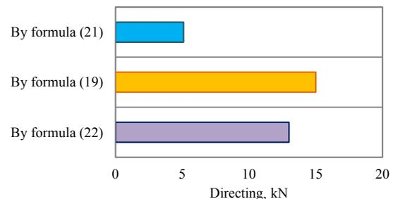
Fig. 7. Comparison of the directing force acting in the first wheel set obtained by different methodologies at train speed of 30 m/s
