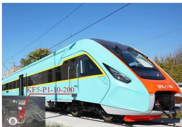
Fig. 8. Schematic of location of strain gauges of KF5-P1-10-200 type in the DPKr-2 train car
