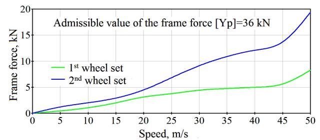
Fig. 2. Dependence of the frame force on motion speed at  $L=15$  m,  $H=0.006$  m
