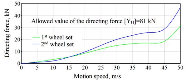
Fig. 6. Dependence of the directing force on the carriage speed at  $L=15$  m,  $H=0.006$  m
