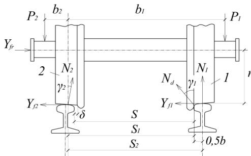
Fig. 5. The forces acting on a wheel set at its interaction with a rail track
