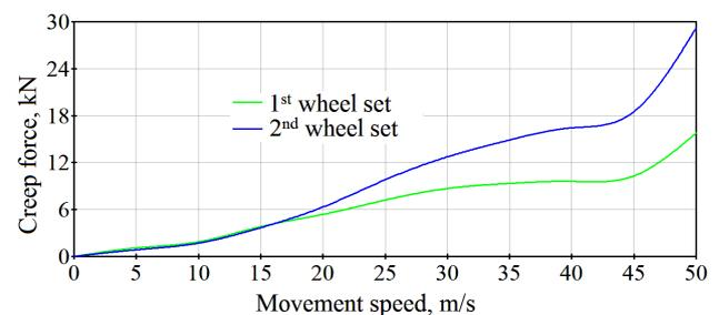
Fig. 4. Dependences of transverse creep forces on the carriage speed at  $L=15$  m,  $H=0.006$  m
