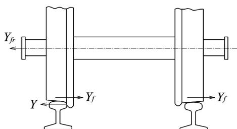
Fig. 1. Horizontal forces acting on the wheel set
