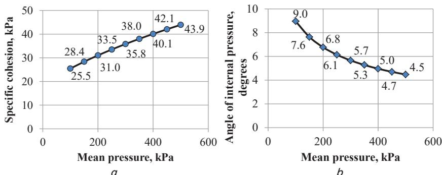
Fig. 3. Relationship between the strength material constants, which are part of the strength conditions by Mohr-Coulomb and A. Shashenko: a – specific cohesion  $c^*$ ; b – angle of internal pressure  $\varphi^*$ . Note: Values of parameters included in the condition of strength by A. Shashenko are equal to:  $c=20$  kPa;  $\varphi=18^\circ$
