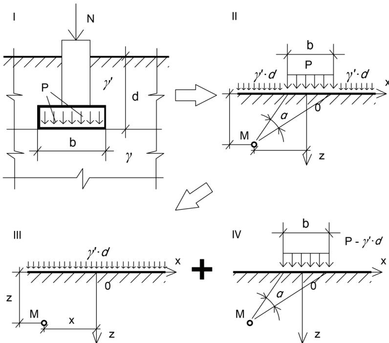
Fig. 1. On determining the initial critical load on soil, as well as the standardized and estimated base resistances: I – system «base – foundation»; II – the corresponding estimation scheme; III, IV – components of the estimation scheme
