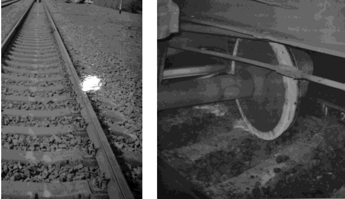
Fig. 1. The traces of the railway wheel motion on the track panel
