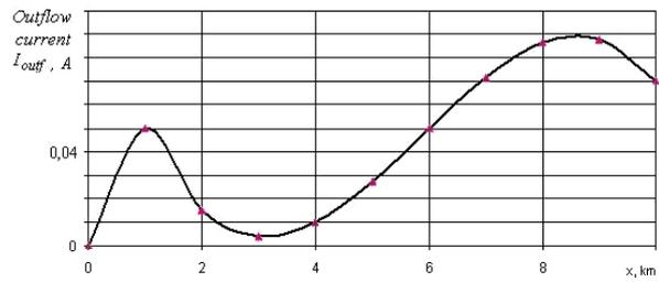
Fig. 4. Dependence of outflow current of 1 A 50 Hz from on coordinate
