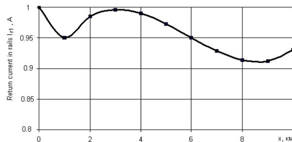
Fig. 5. Dependence of return traction current of 1 A 50 Hz on distance between locomotive and substation
