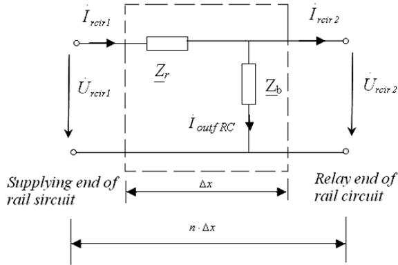
Fig. 2. Equivalent scheme of rail lines
