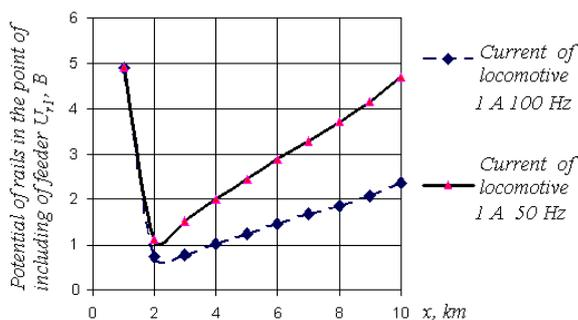
Fig. 6. Dependence of rails' potential on distance between locomotive and substation
