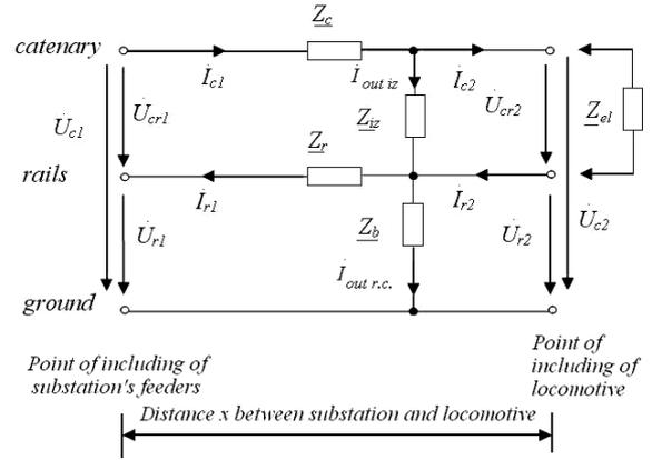
Fig. 1. Equivalent scheme of one-way traction net
