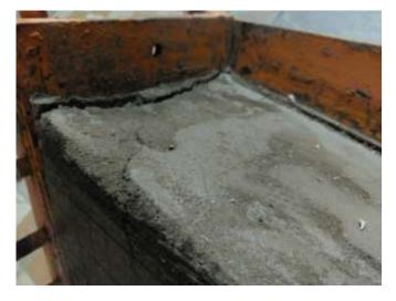
Figure 5. Creation of cracks and separation surfaces, drainage of soil after centrifuge rotation
