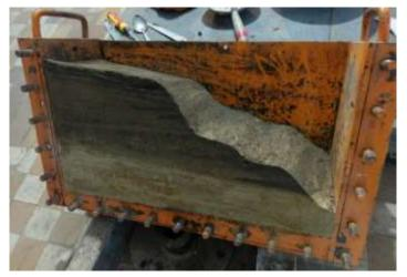
Figure 4 Slope model at scale 1: 100 after cutting of unnecessary soil
