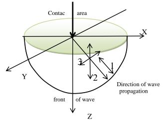
Fig. 1 The scheme of the front of the wave propagation and the directions of oscillation of the particles relative to the direction of propagation of the wave: 1 - direction of propagation of longitudinal waves P; 2 and 3 - directions of propagation of transverse waves S, respectively SV and SH
