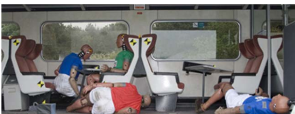
Figure 7. Train Interior Passive Safety – after testing
