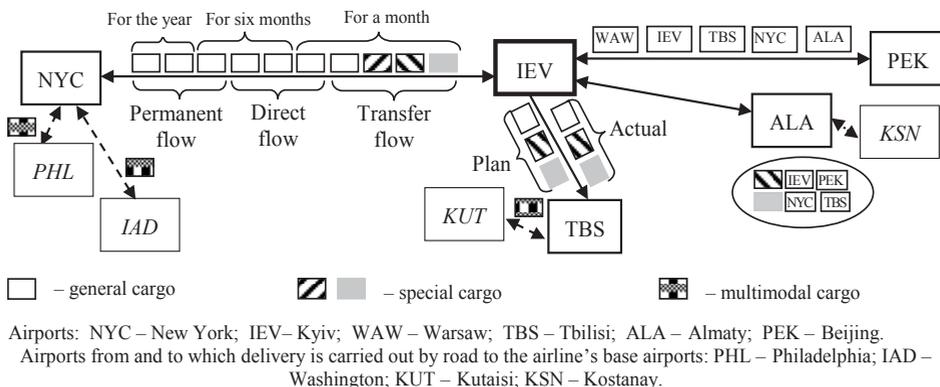
**Fig. 2.** Scheme of cargo flows distribution on the part of the airline network including multimodal flows.
