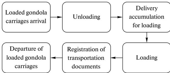
Fig. 2. The procedure for performing operations carriages, incorporated in the technological processes of metallurgical enterprises during the design
