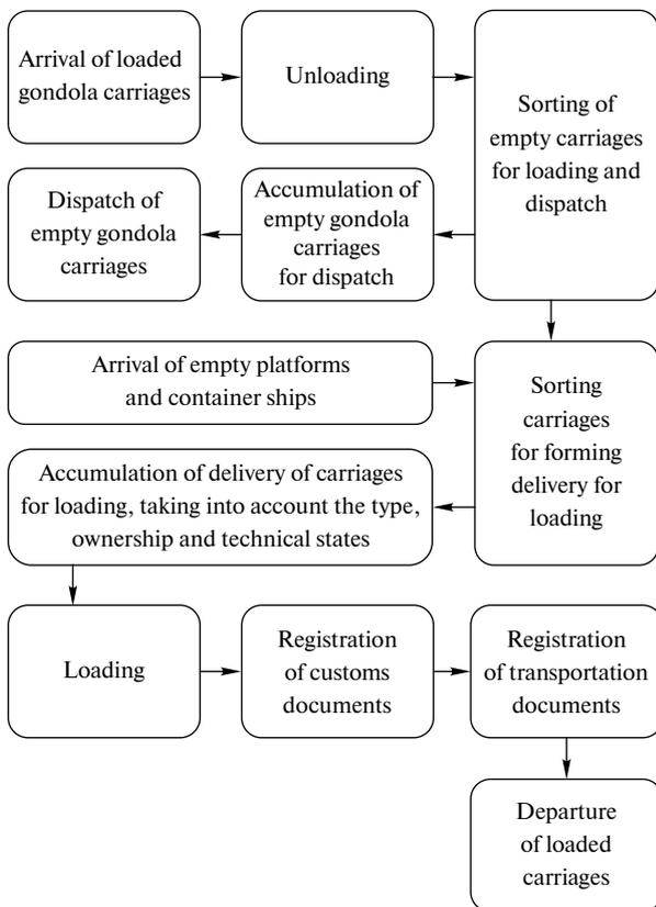
Fig. 3. The actual procedure for performing operations with carriages at metallurgical enterprises
