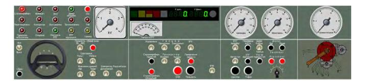
Usage of this hardware-software system allows to teach the operation of the power, support and control circuits of the locomotive in different modes and, it goes without saying, the operation of the train breaking system.
