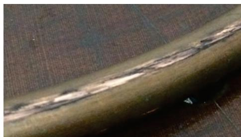
**Fig. 11.** The photo of the surface of the contact wire after testing of the innovative contact strip (sample 1)
