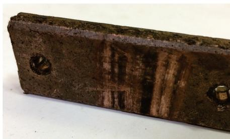
**Fig. 10.** The general view of a fragment of the innovative contact strip (sample 1)
