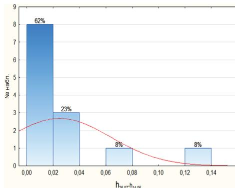
**Fig. 4.** The results of processing the values of the difference in heights of the left contact wire in the even direction
