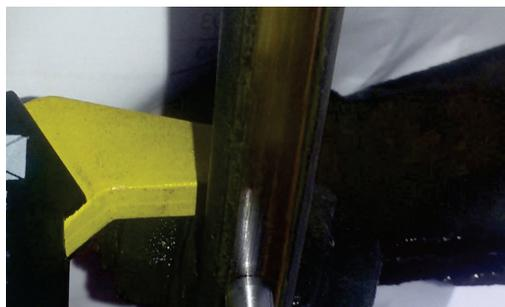
**Fig. 8.** The working surface of the contact wire in one of the control points, as of March 30, 2017
