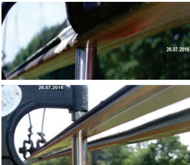
**Fig. 6.** The working surface of the contact wire at one of the control points, as of July 26, 2016
