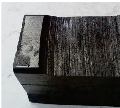
**Fig. 16.** The general view of a fragment of the traditional contact strip (sample 9)
