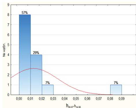
**Fig. 3.** The results of processing the values of the difference in heights of the left contact wire in the odd direction
