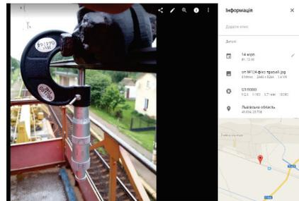
**Fig. 2.** Screenshot of a photo with measurements of the height of the contact wire
