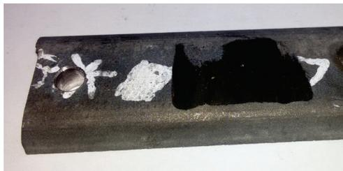
**Fig. 12.** The general view of a fragment of the traditional contact strip (sample 3)
