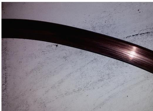
**Fig. 17.** The photo of the surface of the contact wire after testing of the traditional contact strip (sample 9)
