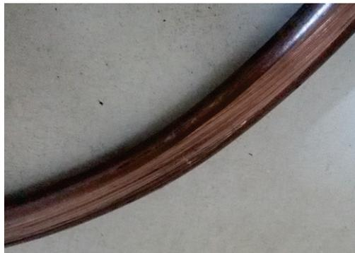
**Fig. 15.** The photo of the surface of the contact wire after testing of the traditional contact strip (sample 8)
