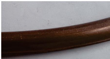
**Fig. 13.** The photo of the surface of the contact wire after testing of the traditional contact strip (sample 3)
