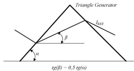
Fig. 2. The principle of the reference-input signal formation to ensure the stability of the system
