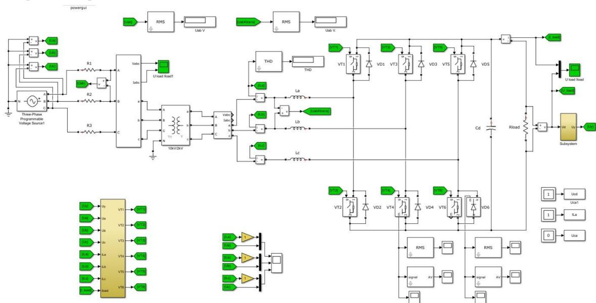
Fig. 5. Simulation model of an active rectifier with a triangular method of forming PWM in Matlab Simulink
