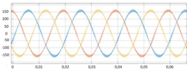
Fig. 8. Oscillograms of input current
