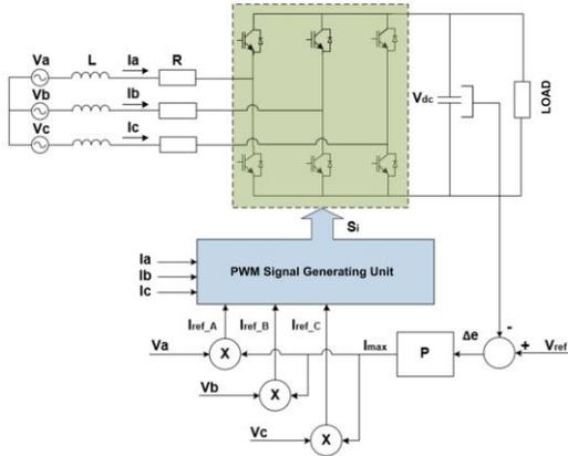
Fig. 3. Active Rectifier Control System
