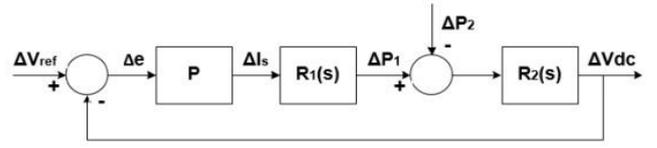
Fig. 4. Control System of Active Voltage Rectifier
