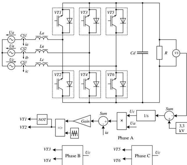
Fig. 1. Full-bridge three-phase active rectifier scheme
