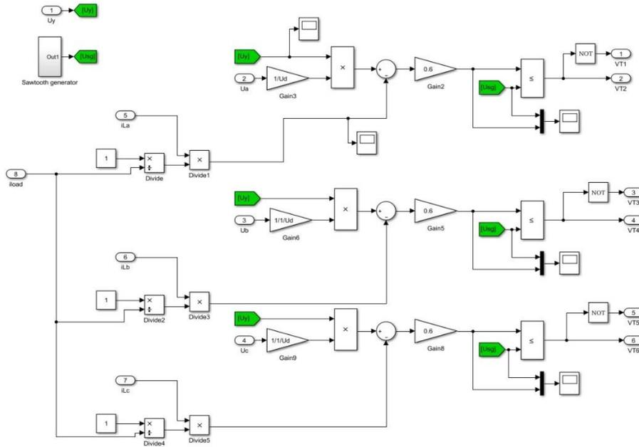
Fig. 6. Control system of the converter in the Matlab Simulink environment
