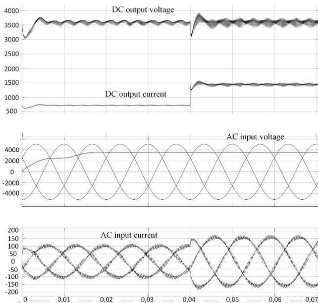
Fig. 11. Oscillograms of input and output current and voltage with an abrupt load change
