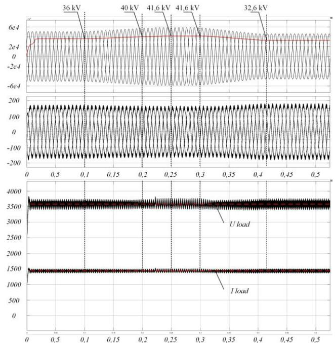
Fig. 9. Oscillograms of the output current and voltage of the contact network with a change in the input voltage level of the supply network.
