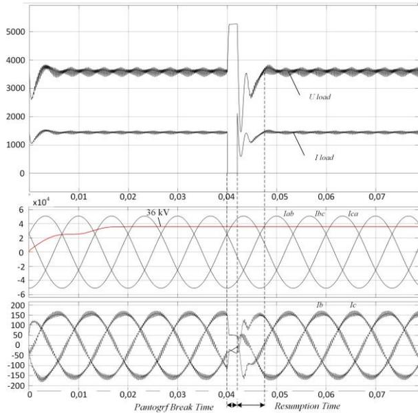
Fig. 10. The result of the experiment mode of the pantograph bouncing
