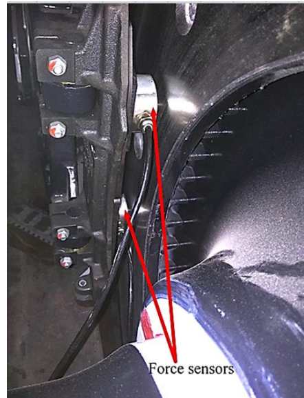
Figure 2. Installation of force sensors in determining the force of pressing the pad.
