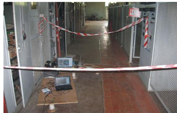
**Fig. 2.** Location of measurement equipment into the 3.3 kV distributive device of traction substation № 19.
