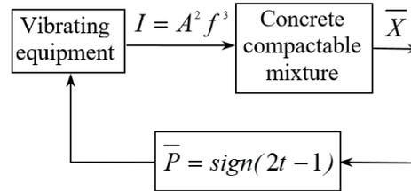
**Figure 1** Block diagram of the concrete mixture vibrations compaction control with feedback, where:  $I$  - is the intensity of compaction,  $A$  - is the vibrations amplitude of the vibrations device,  $f$  - is the vibrations frequency of the vibrations device
