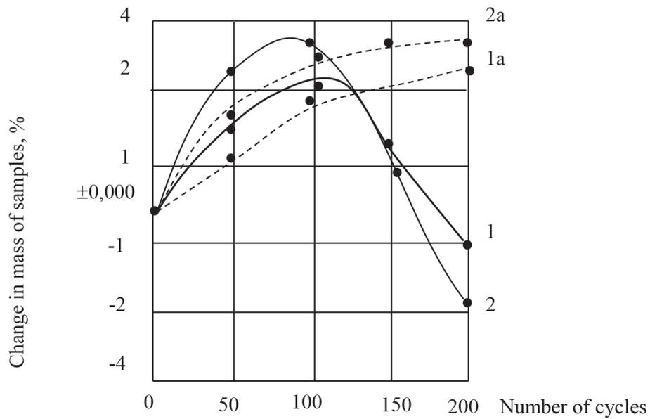
**Figure 3** The mass of concrete samples depending on the duration of hardening, the number of freezing and thawing cycles: 1 - for samples formed with optimal control and freezing-thawing; 1a - the same, for control samples; 2 - for samples molded according to the traditional mode (with constant vibrations intensity) and subjected to freezing-thawing; 2a - the same, for control samples
