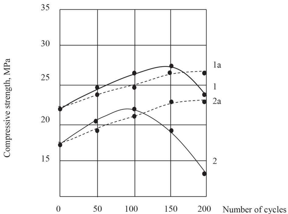
**Figure 4** Compressive strength of concrete samples depending on the duration of hardening, the number of freezing and thawing cycles: 1 - for samples formed with optimal control and freezing-thawing; 1a - the same, for control samples; 2 - for samples molded according to the traditional mode (with constant vibrations intensity) and subjected to freezing-thawing; 2a - the same, for control samples
