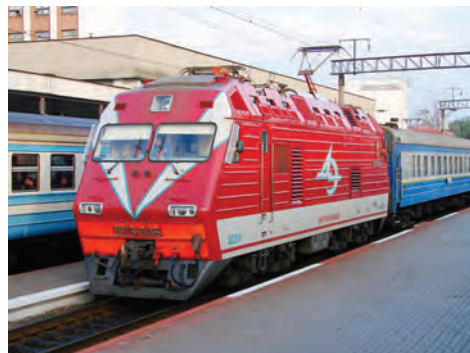
Fig. 3. DS3 one-section electric locomotive
