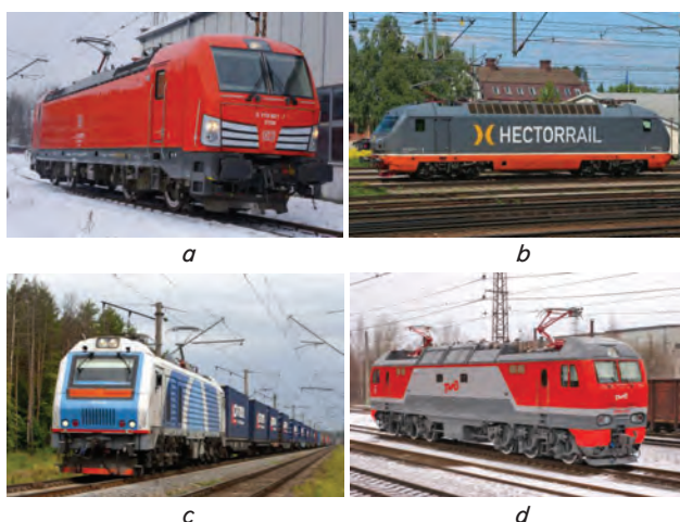
Fig. 2. Modern one-section electric locomotives: a – Vectron (Germany); b – Taurus Rh242 Hectorrail (Sweden); c – BKG2 (China); d – EP2 (Russia)
