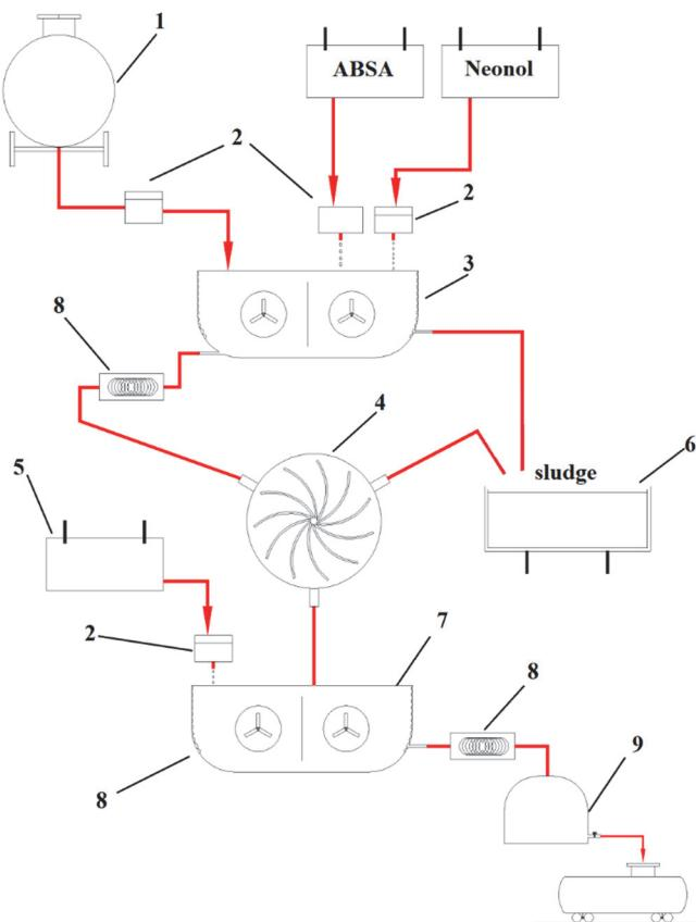
**Fig. 1.** Scheme for treatment of discarded waste oil; 1 – balance tank, 2 – dosing pumps, 3 – first-stage mixer with heating, 4 – centrifuge, 5 – additive storage tank, 6 – sludge collector, 7 – second-stage mixer, 8 – pumps, 9 – storage tank for restored oil
