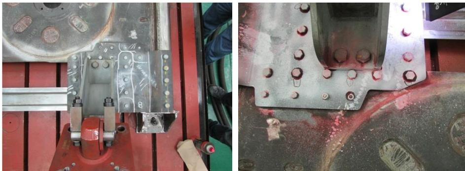
**Figure 5.** Marking of places and results of intermediate penetrant control zone 1.
