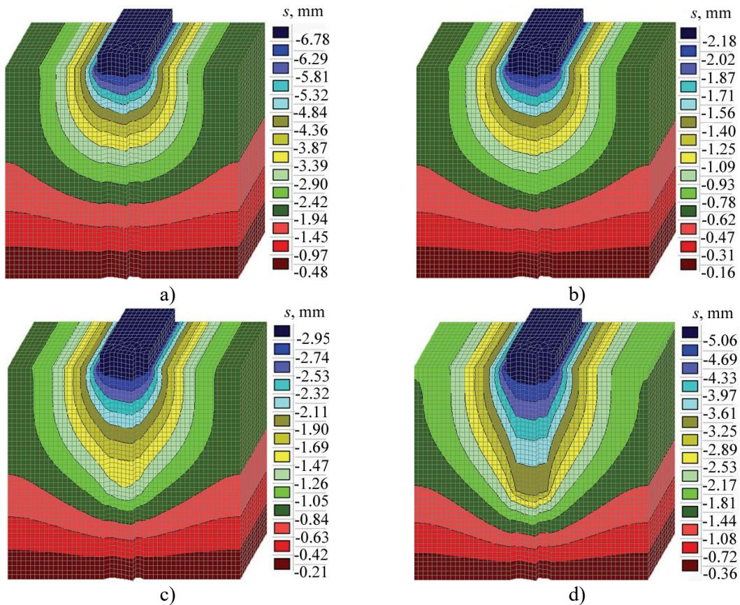
**Figure 2.** Characteristic isolines and isofields of vertical displacements  $s$  (mm) in finite-element models: a) unsupported by micropiles,  $E_s = 5$  MPa; b)  $E_{mp} = 30$  MPa,  $E_s = 15$  MPa; c)  $E_{mp} = 60$  MPa,  $E_s = 10$  MPa; d)  $E_{mp} = 90$  MPa,  $E_s = 5$  MPa.
