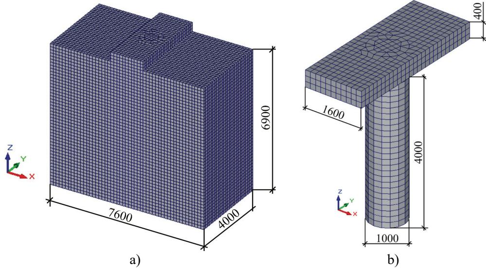
**Figure 1.** The finite-element model of the geotechnical system "soil base–micropile" with the strip foundation: a) a general view; b) a fragment of the model – foundation with the micropile.
