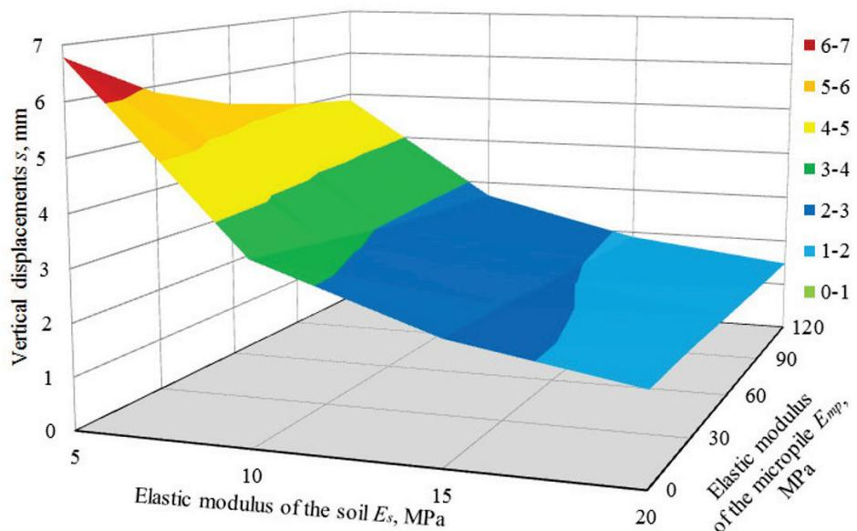
**Figure 4.** The regularity of vertical displacements from the elastic modulus of the soil base and the micropile.
