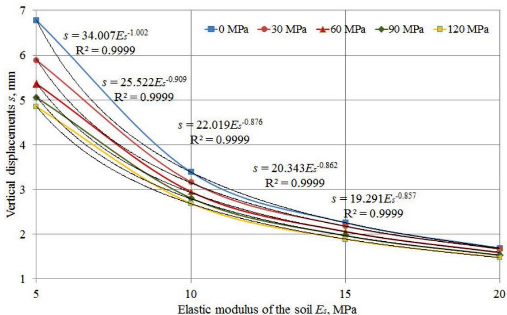
**Figure 3.** The regularity of vertical displacements from the elastic modulus of the soil base.
