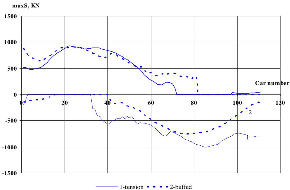
Fig. 3 Distribution of longitudinal forces maximum values along the preliminary tension and buffed trains consisted of tank-cars at the emergency braking from the speed of 20 km/h by only the second locomotive (through braking pipe).
