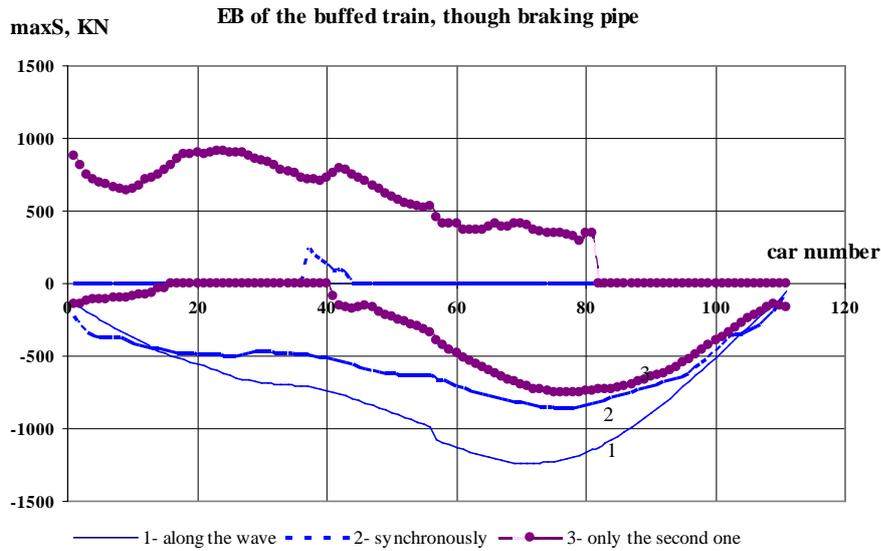
Fig. 4 Distribution of the longitudinal forces maximum values along the train at the emergency braking of the preliminary buffed trains made-up from tank-cars for various ways of brakes control.
