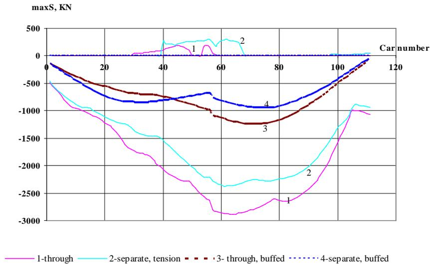
Fig.2. Distribution of the maximum longitudinal forces along the train composed from the tank-cars at the emergency braking by the lead locomotive when the second locomotive is situated in the middle of the train and is braking by the discharge wave of the braking line for the preliminary tension (solid curves) and buffed (dot curves) trains.
