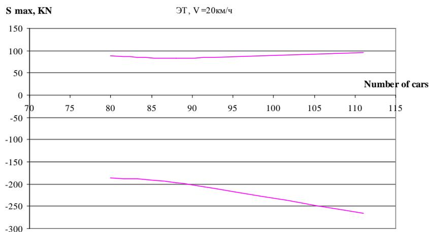
Fig. 1. Dependence of the highest longitudinal forces in the train on the number of tank-cars at the emergency braking by the lead locomotive.
